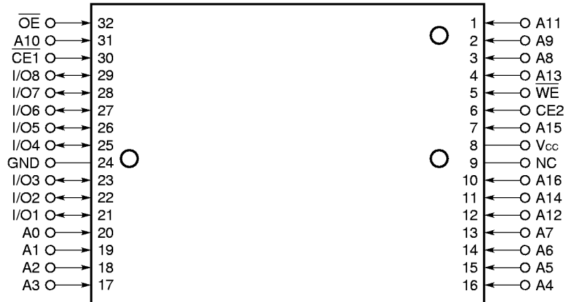
32-pin Plastic TSOP (I) (8 × 13.4mm) (Reverse bent) [μPD431000AGU-9KH]
